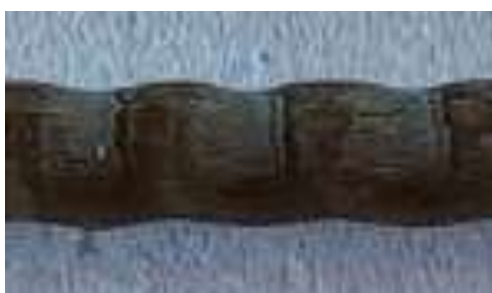
Figure 5. Crushing of the resin and fibre of BFRP bars (25 °C to 85 °C)
