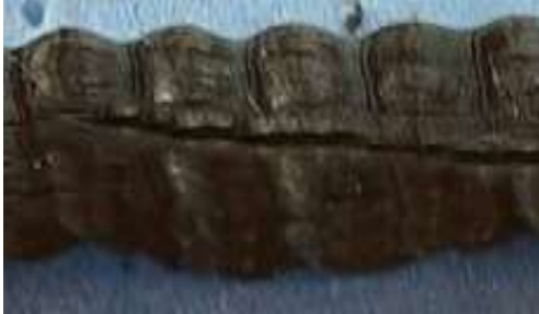
Figure 7. Interlaminar shear failure of the 12.0 mm and 14.0mm BFRP bars (25 °C to 85 °C)
