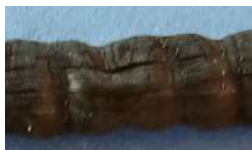
Figure 6. Interlaminar shear failure of BFRP bars (25 °C to 85 °C)
