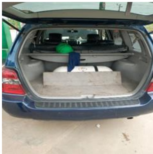
Figure 1: The trunk of the Toyota Highlander 2010 showing the CNG cylinder.
